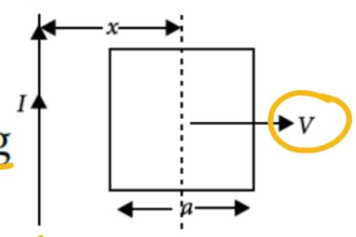
in the figure. The frame moves to the right with a constant velocity 'V'. The emf induced in the frame will be proportional to
