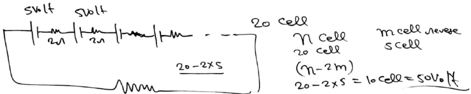
⇒ If 5-cell connected opposite polarity in out of 20-cell.
