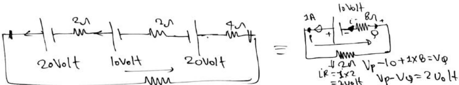
(i)  $I_{\text{net}} \text{ in Ckt} = \frac{E_{\text{net}}}{R_{\text{net}}} = \frac{20}{10} = 2 \text{ Amp}$        $E_{\text{net}} = E_1 + E_2 + E_3$
